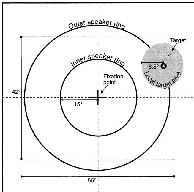
Figure 1. Diagram of the speaker setup for both experiments.
